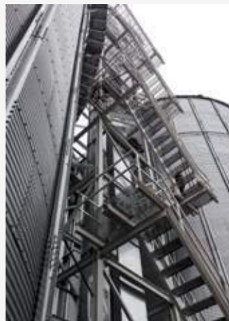
Country: Latvia Project: Saldus Grauds Year: 2017 Bucket elevator E500, 500 t/h Bucket elevator E80, 80t/h x 5 Chain conveyor K100, 100 t/h x 2 Chain conveyor K100, 80t/h x 3 Flight conveyor with bend S500L, 500 t/h 2-way valves Service tower for bucket elevator.
