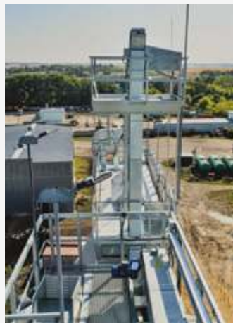
Country: Russia Year: 2020 Chain conveyor K120, 100t/h x4 Bucket elevator E80, 100t/h x 3 Flight conveyor S100, 100t/h Accessories Continuous Flow Dryer GXL11, 60 t/h (wheat).
