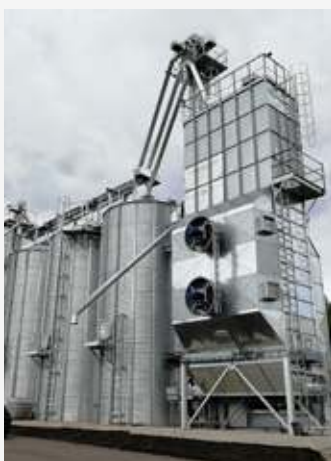
Country: Estonia Year: 2018 Bucket elevator E80, 80 t/h x 2 Batch dryer BXL76 Chain conveyor K100, 100 t/h.
