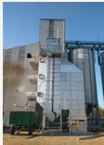
Country: Latvia Project: farm Siecini Year: 2017 Continuous flow dryer GL6, 21 t/h (wheat) Chain conveyors K100, 100 t/h Bucket elevators E80, 80 t/h.
