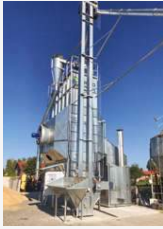
Country: Poland Year: 2022 Mobile grain dryer MD2x3 Air cleaning unit PA100.
