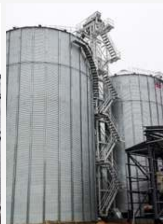
Country: Latvia Project: Saldus Grauds Year: 2017 Bucket elevator E500, 500 t/h Bucket elevator E80, 80t/h x 5 Chain conveyor K100, 100 t/h x 2 Chain conveyor K100, 80t/h x 3 Flight conveyor with bend S500L, 500 t/h 2-way valves Service tower for bucket elevator.
