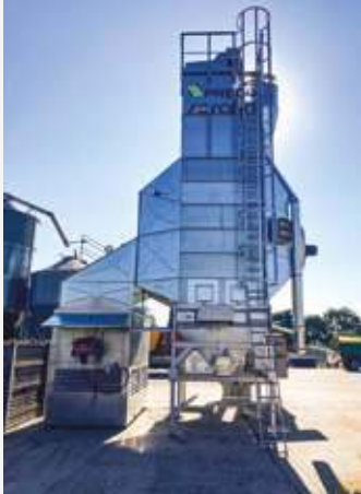
Country: Poland Year: 2022 Mobile grain dryer MD2x3 Air cleaning unit PA100.
