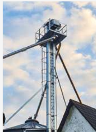
Country: Austria Year: 2022 Flight conveyor S80, 60t/h Bucket elevator E80, 60t/h Belt conveyor L500, 52m, 60t/h Intake pit PB.
