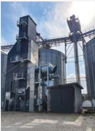
Country: Germany Year: 2023 Chain conveyor K120, 120t/h Flight conveyor S150, 120t/h Bucket elevator E150, 120 t/h Chain conveyor K40, 30t/h Continuous grain dryer GL10 3-way and 2-way valves.
