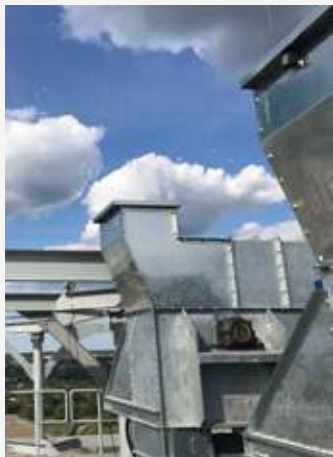
Country: Ukraine Project: Zorya Podoliya Year: 2016 Chain conveyors K300, 250 t/h Bucket elevators E300, 250 t/h.
