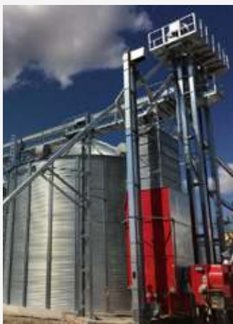
Country: Lithuania Year: 2019 Bucket elevator E80, 80t/h x 3 Chain conveyor K100, 80t/h x 3 2-way valves, grain brakes.
