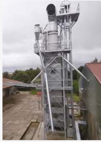
Country: Germany Year: 2021 Project: grain and maize reception, processing and storage Chain conveyor K60, 60t/h Flight conveyor S60, 60t/h Bucket elevator E80, 60 t/h Grain intake pit Continuous grain dryer GM-6 CTF.
