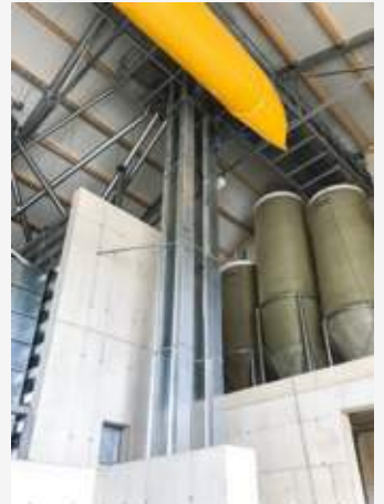
Country: Austria Year: 2022 Flight conveyor S80, 60t/h Bucket elevator E80, 60t/h Belt conveyor L500, 52m, 60t/h Intake pit PB.
