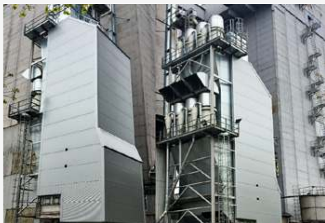
Country: Latvia Year: 2017 Flight conveyor with bend 45° S200L, 150 t/h Chain conveyor K200, 150 t/h Bucket elevator E150, 150 t/h Continuous Flow Dryer GXL13, 65 t/h (wheat).
