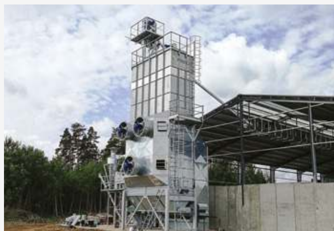
Country: Latvia Year: 2019 Batch dryer BXL64 Chain conveyor K60, 60 t/h x 2 Flight conveyor with bend S80L60, 60 t/h.
