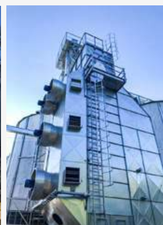
Country: Latvia Project: LIS Year: 2019 Continuous flow dryer GL7, 25 t/h (wheat) Chain conveyor K100, 60 t/h Drive-over intake pit PB3.5x10m Flight conveyor S80L with bend, 80 t/h x 3 Chain conveyor K100, 80t/h Flight conveyor S80L with bend, 60 t/h Bucket elevator E80, 60 t/h Chain conveyor K100, 80t/h Chain conveyor K100, 100 t/h.
