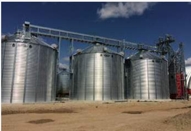
Country: Lithuania Year: 2019 Bucket elevator E80, 80t/h x 3 Chain conveyor K100, 80t/h x 3 2-way valves, grain brakes.
