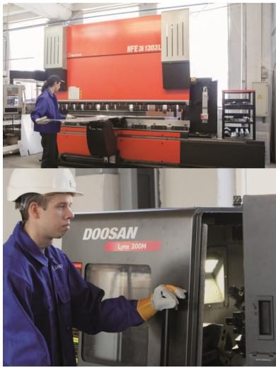
CNC Sheet metal bending
